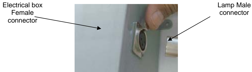
Figure 2. Lamp connector connection with electrical box
