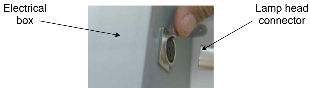
Figure 8. Lamp lead connection with electrical box
